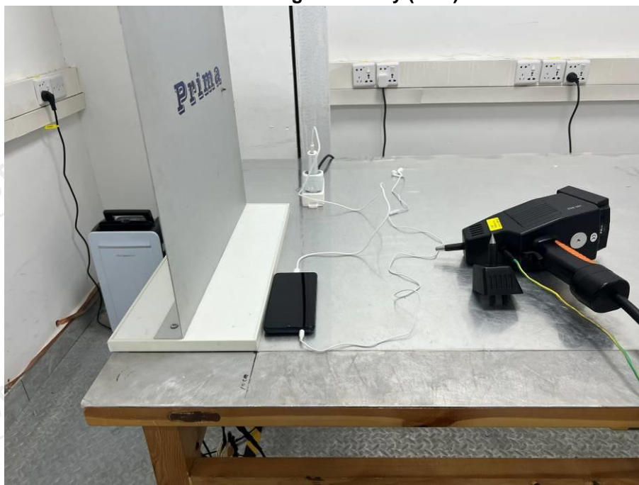
Electrostatic discharge immunity (ESD) test view
