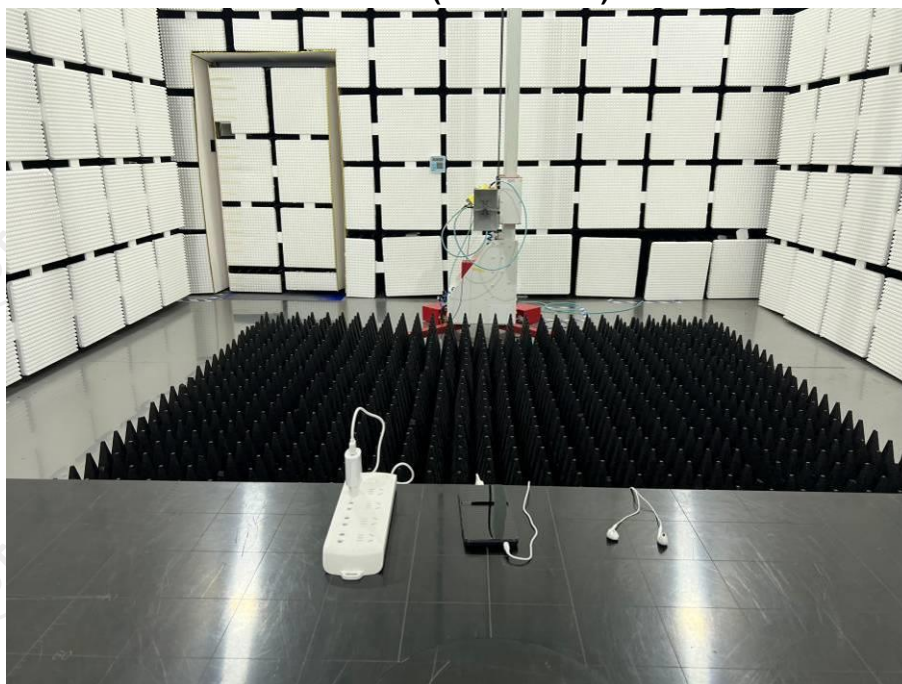
Radiated emission (1 GHz-6 GHz) test view
