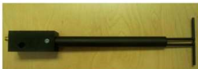
Figure 1 – MVG COMOSAR Validation Dipole
