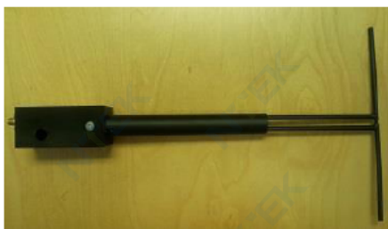
Figure 1 – MVG COMOSAR Validation Dipole
