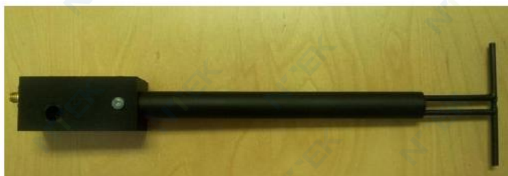
Figure 1 – MVG COMOSAR Validation Dipole
