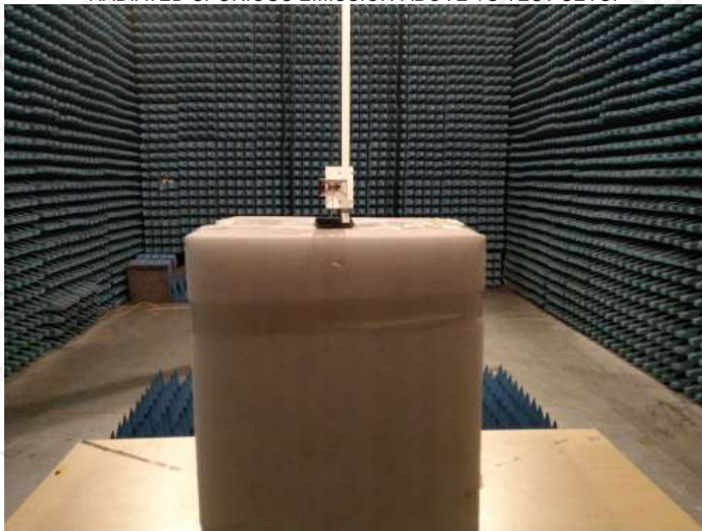
RADIATED SPURIOUS EMISSION-ABOVE 1G TEST SETUP
