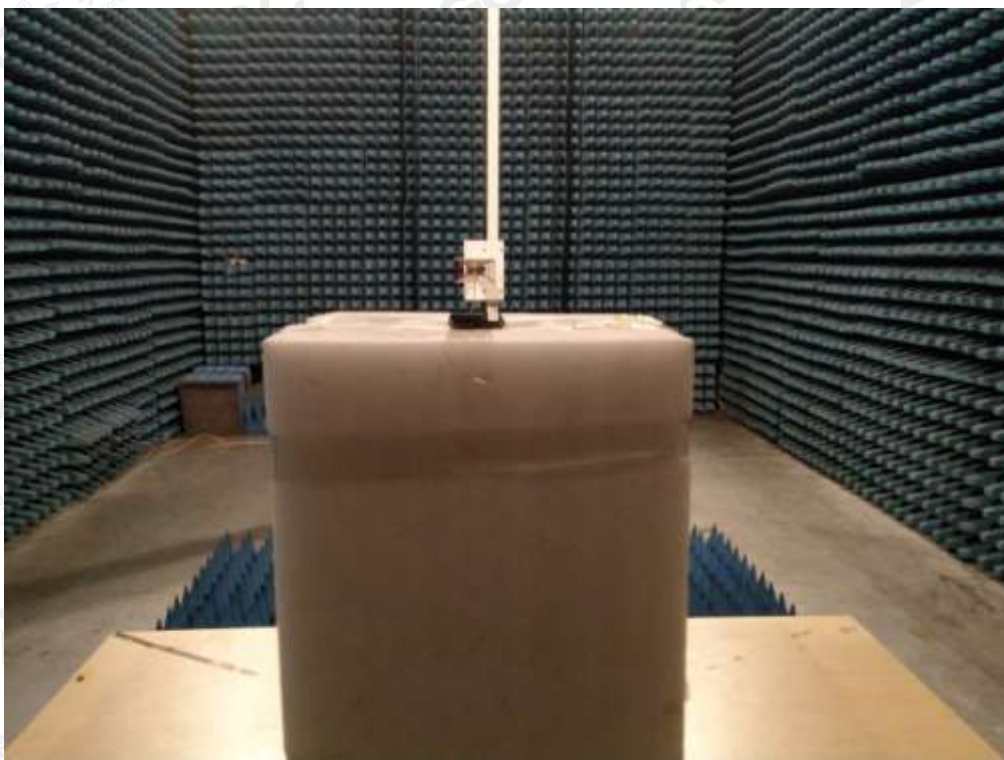
RADIATED SPURIOUS EMISSION-ABOVE 1G TEST SETUP
