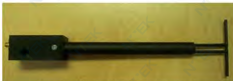
Figure 1 – MVG COMOSAR Validation Dipole
