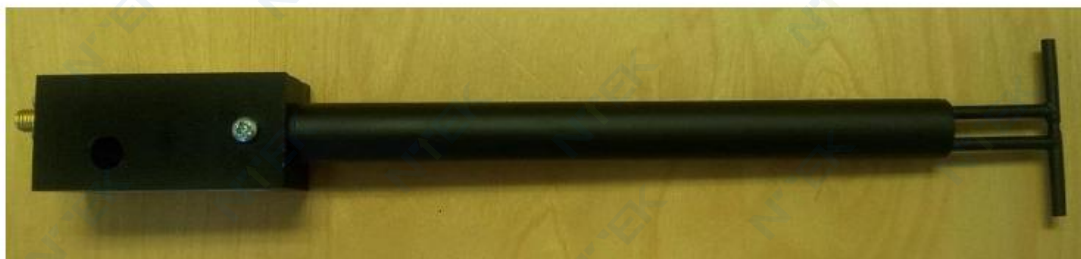
Figure 1 – MVG COMOSAR Validation Dipole
