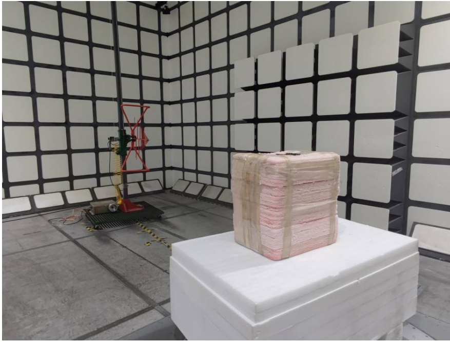
Radiated Spurious Emissions Test View (Above 1GHz)
