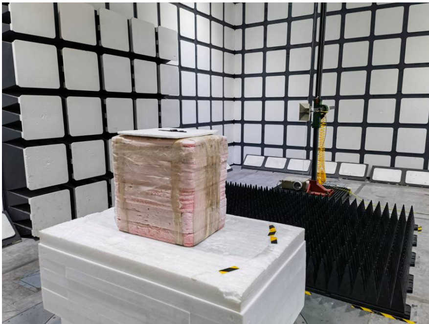
Radiated Spurious Emissions Test View (Above 1GHz)
